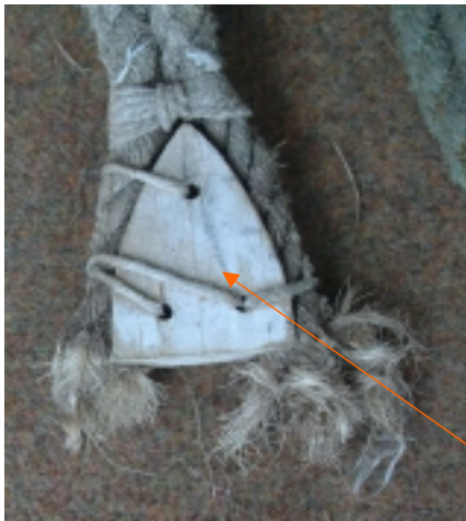
Photo 3 Close-up of right-hand fail zone
