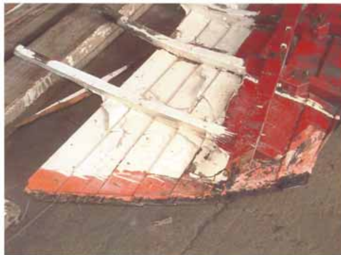
Figure 3. Foot of bow, with scarf joint in stem, base of Samson post, and missing keel
