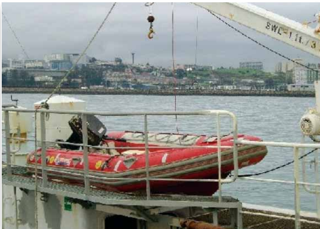
Rescue boat in stowed position. Note the lowering gear is not connected and the boat consequently is not ready for immediate use.
