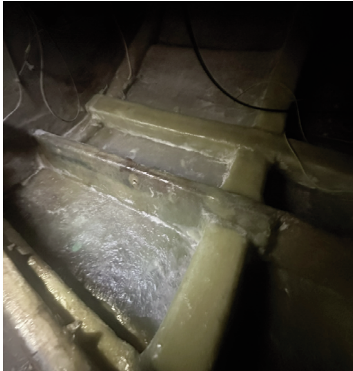
Figure 8: Fibreglass repairs to the hull with extra stiffeners added.
