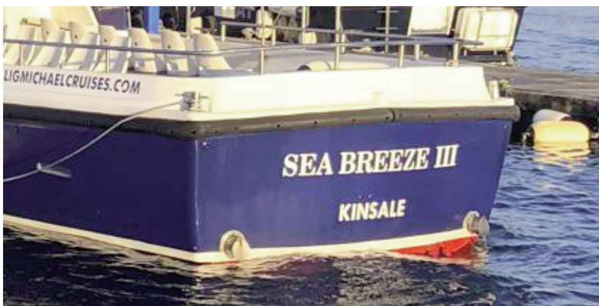
Figure 6: Exhaust arrangement on MV Sea Breeze III.
