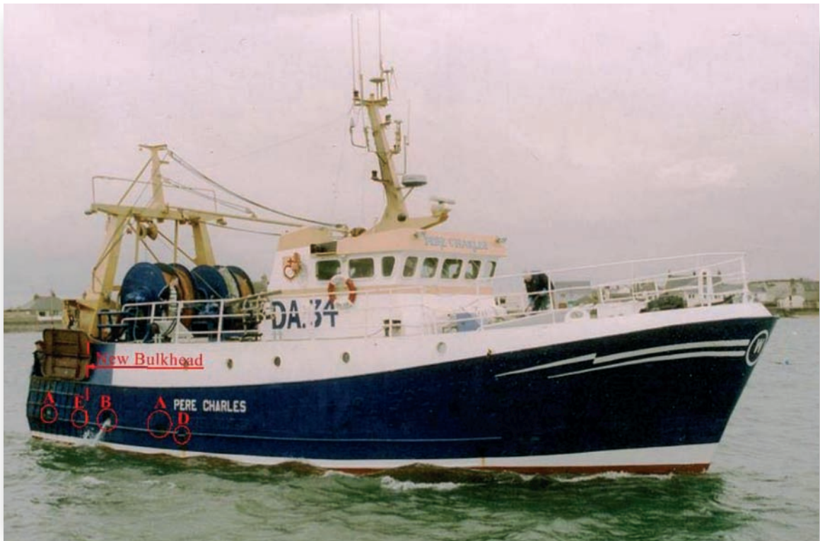
Photograph 1 - Freeing Ports on Starboard Side.
