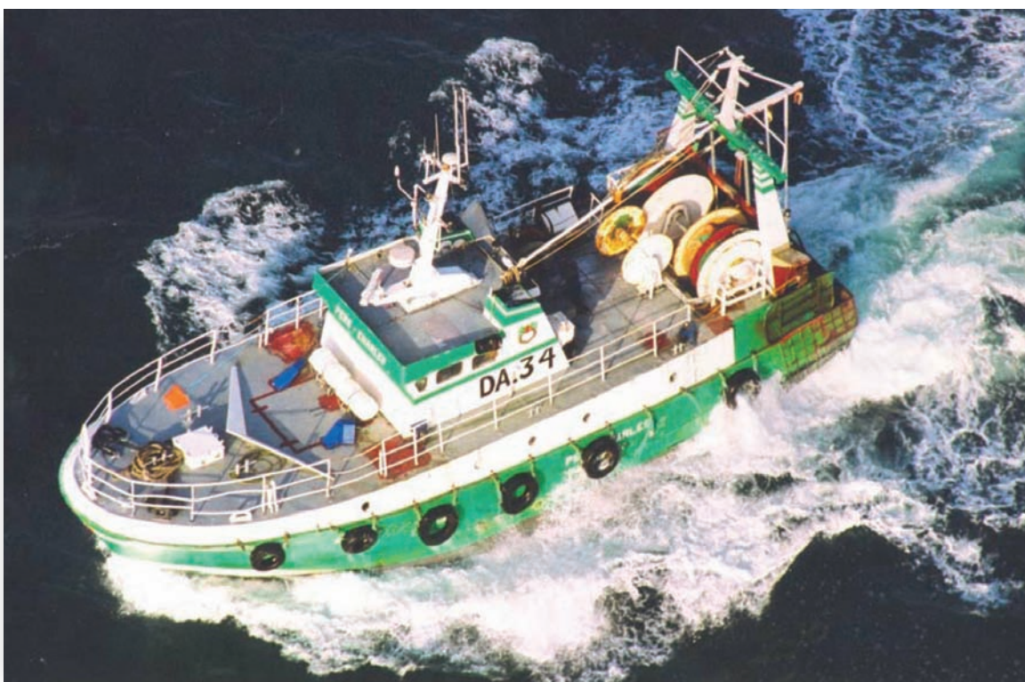
Photograph 12 - Pere Charles at sea - note freeing ports at after fender are submerged.
