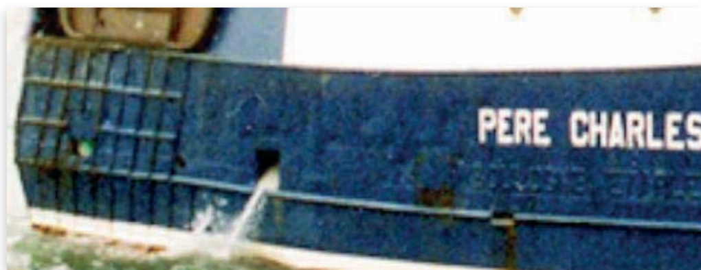
Photograph 1a - Enhanced Photograph 1 - Freeing Ports on Starboard Side.
