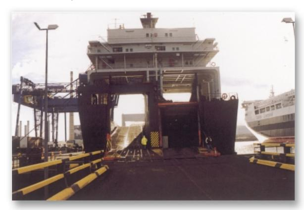
A view from the head of the linkspan looking onto the stern of "Merchant Bravery". The raised aft mooring deck can be seen over the port stern opening leading up to the weather deck. Personnel can be observed walking on the ship's ramp/door that is resting in position on the linkspan.
