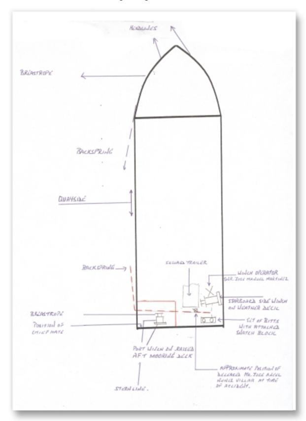
Plan of the aft section of "Merchant Bravery" with captions to the aft mooring deck area.
