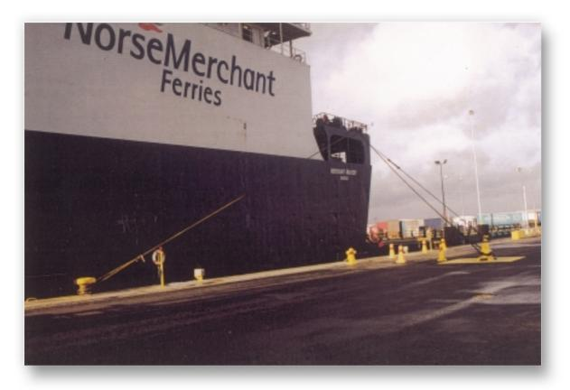
"Merchant Bravery" secured port side to Berth 53. Seen in the photograph is the backspring leading forward and the breast and stern lines secure onto shore bollards.
