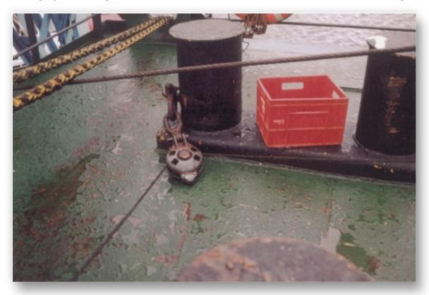
The actual method used to connect the snatch block to the mooring bitts.
