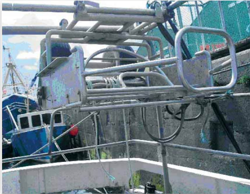
Photo No. 3: The pot stacker. Two rope ends can be seen trailing from the hauling drum. This was the means by which Mr. Egan was recovered.
