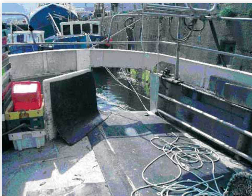
Photo No. 1: Working deck and open stern door on the MFV "MDAC".
