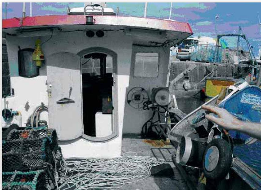
Photo No. 2: View of the wheelhouse from aft. Mr. Egan was standing on the starboard (right side) of the wheelhouse. The pot ropes have been disturbed after Mr. Egan was pulled over the side but the potential for a fisherman to be snared can be clearly seen from this photograph.
