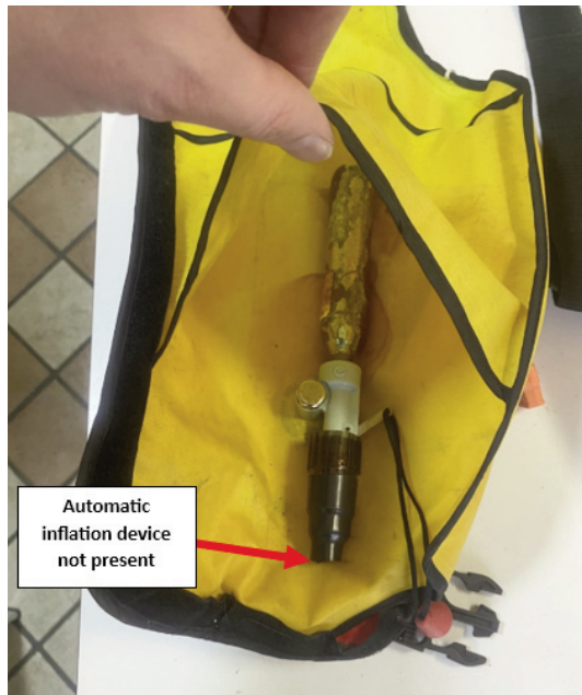
Photograph No. 6: Showing the condition of the PFD inflation device.
