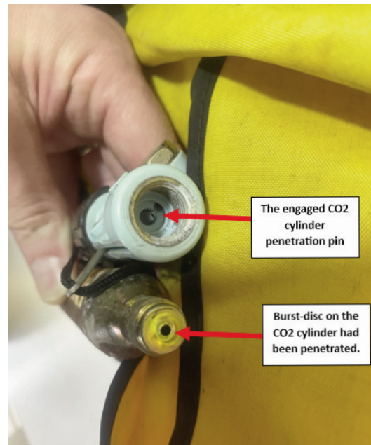
Photograph No. 7: The Casualty's PFD showing the discharged CO2 cylinder.
