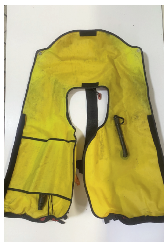
Photograph No. 5: Internal condition of the Casualty’s PFD on inspection.
