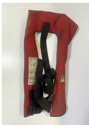
Photograph No. 4: The external condition of the Casualty’s PFD.
