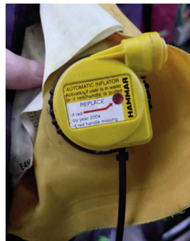
Photograph No. 9: Three of the four onboard PFDs in poor condition with one of the activation units over 18 years out of service.
