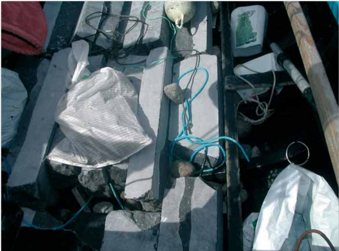
Ballast wedged in place between stringers in the bottom of the hull.
