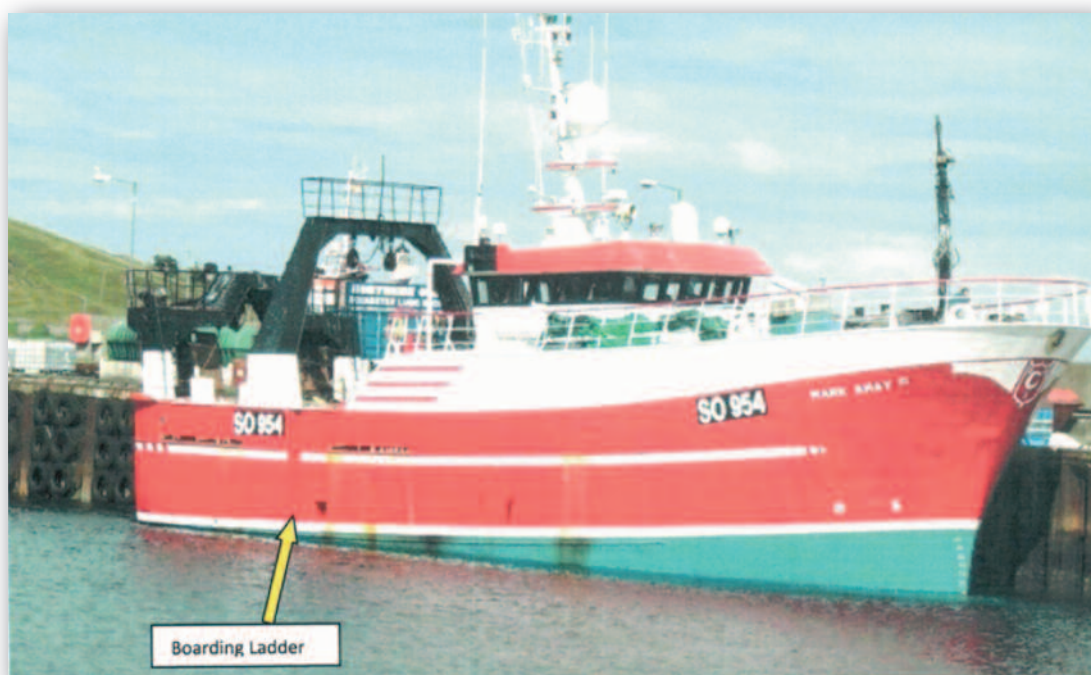
Appendix 9.6 Photo of Vessel Showing Boarding Ladder.
