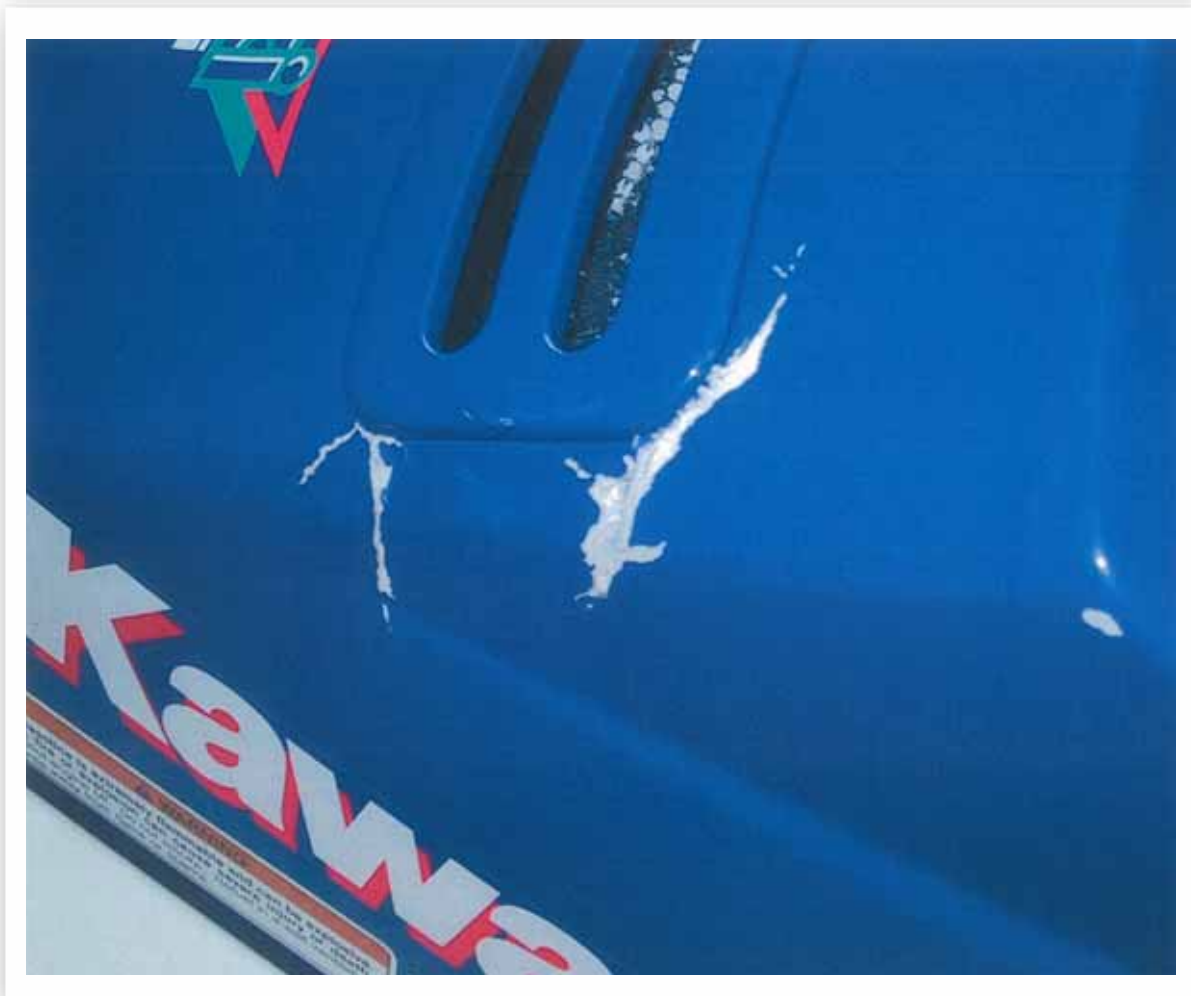
Appendix 8.8 Photograph showing the damage caused in portside upper side.
