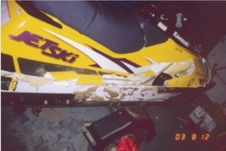
FIGURE 9 DAMAGE TO STARBOARD SIDE TOPSIDE TO HULL JOINT
