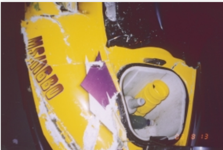
FIGURE 7 DAMAGE TO TOPSIDE COWLING
