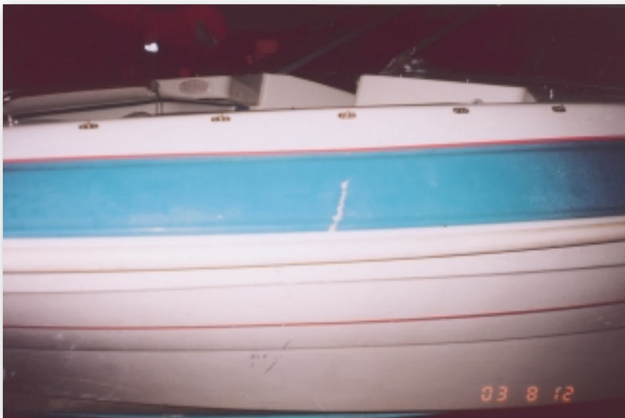
FIGURE 2 DAMAGE TO HULL & DECK JOINT
