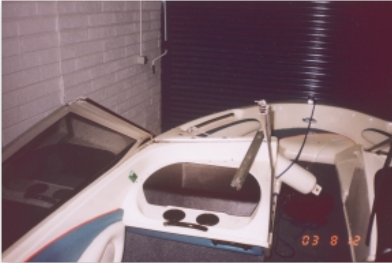
FIGURE 3 DAMAGE TO WINDSHIELD
