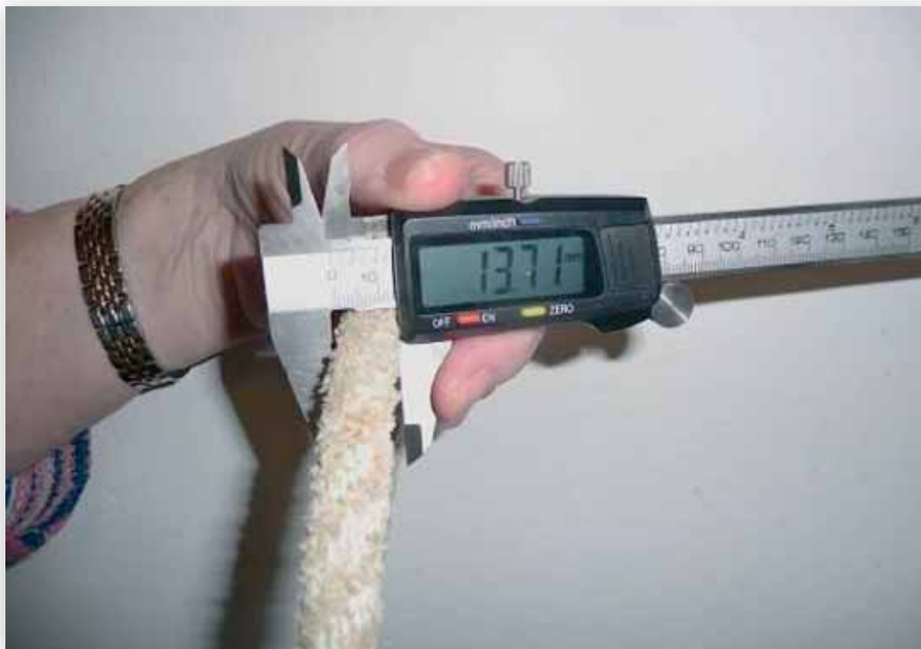
c) Pot rope 13.71mm Diameter.
