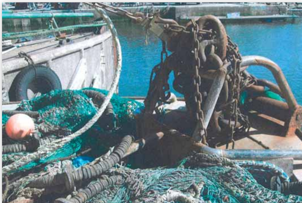
Photo 2 - View to starboard over net bin with clump secured in its cage on bulwark rail and securing senhouse slip in place.
