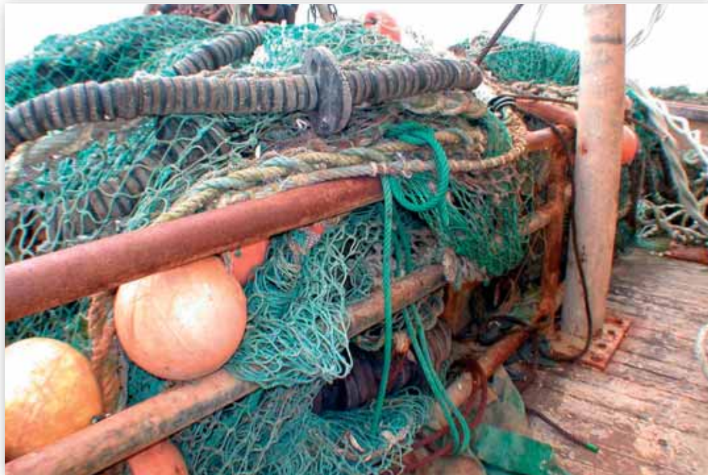
Photo 1 - Net bin arrangements viewed to port with position of clump visible aft.
