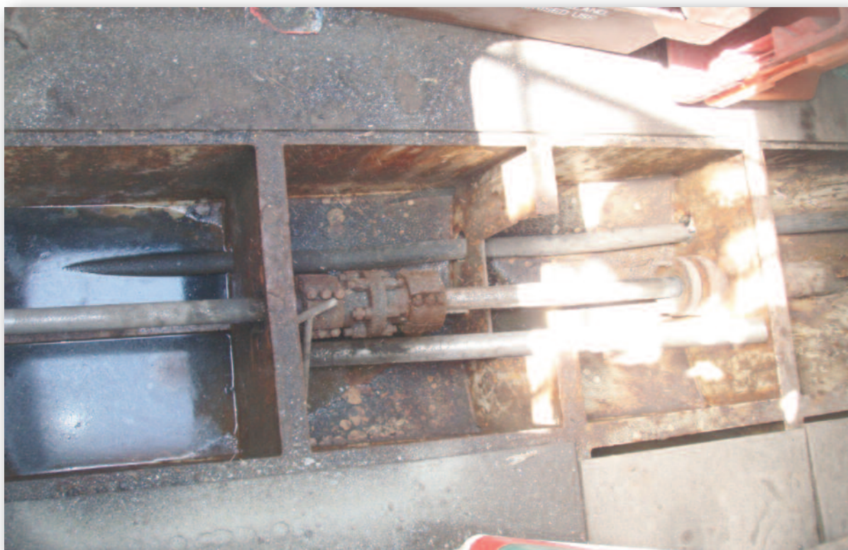
Photo 2: Sole boards in fish hold lifted. Casualty's leg caught in coupling of the shaft.
