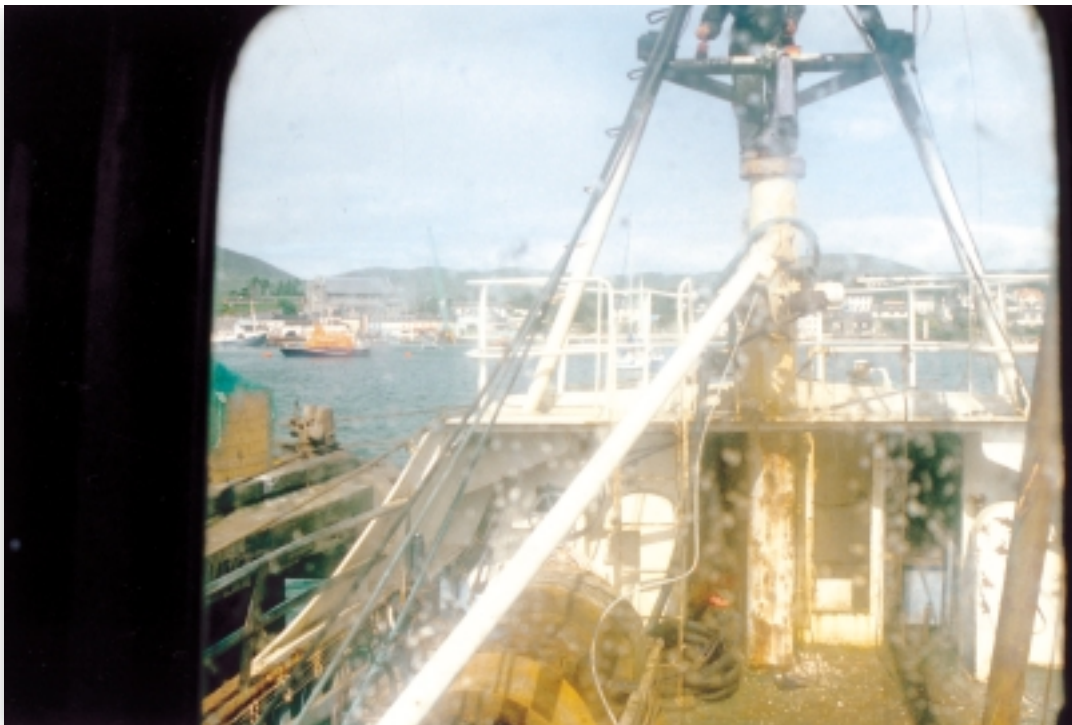
Visibility through forward facing window to the port side of wheelhouse 'Princess Grainne'.
