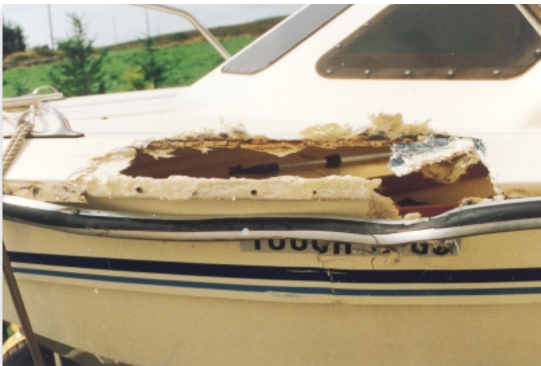
Damage sustained to port side of 'Touch-n-Go'.
