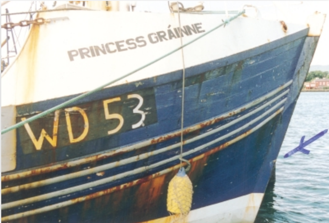
Arrow points to impact scuff marks where 'Princess Grainne' made contact with 'Touch-n-Go'.
