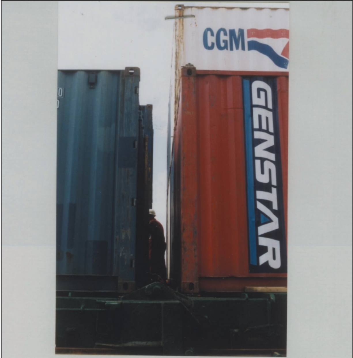
Photograph “a” shows the stowage arrangement that provides for an athwartships 18 inch corridor at 40 foot intervals between section 2 and section 3 . The photograph is taken from the quayside port side of the ship. See also photograph “g”
