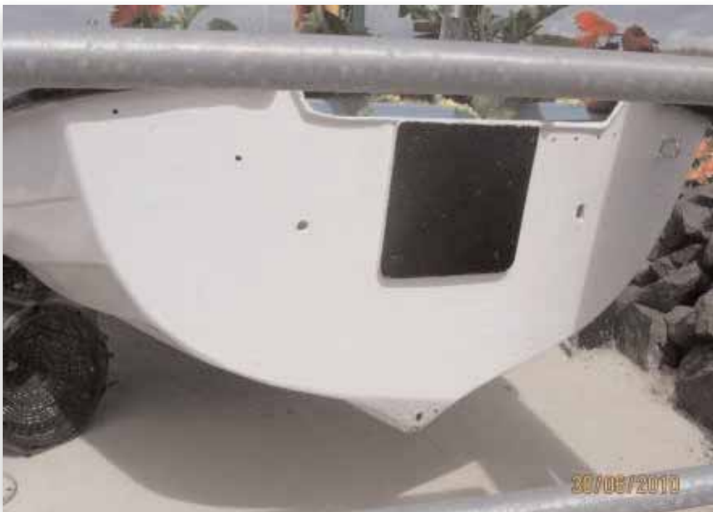
(b) Transom drain holes almost at same level as second strake from gunwhale.
