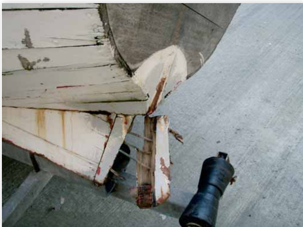
(b) Damage to skag.
