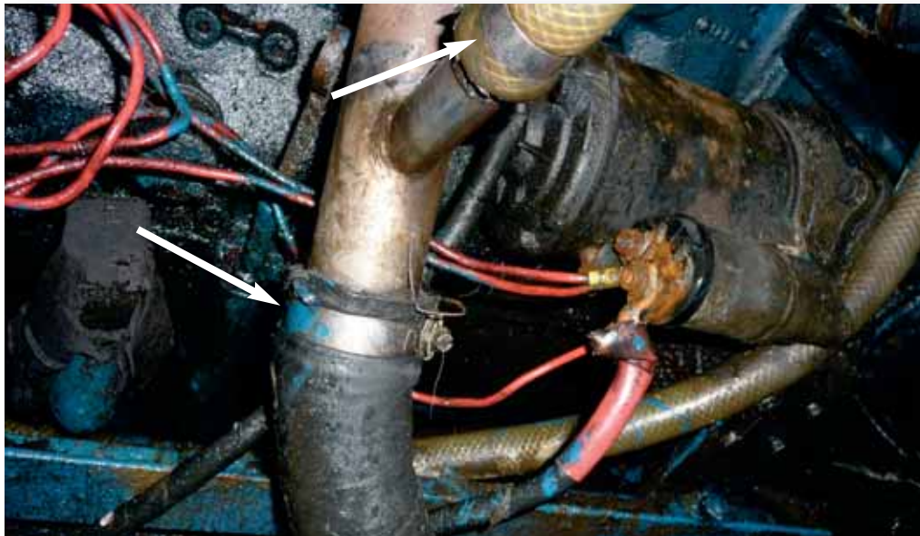
Single Hose Clips on Exhaust System
