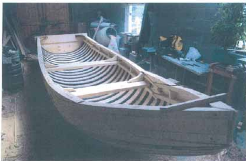
Figure 4, shows the currach completely planked and ready for its fiberglass coating.
