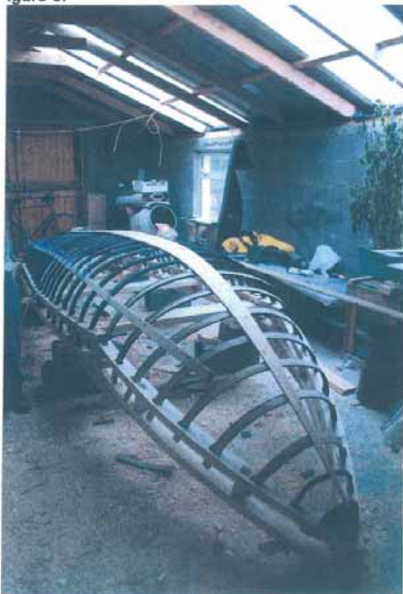
Figures 2 & 3 show the first plank attached and the hull partially covered with planks.
