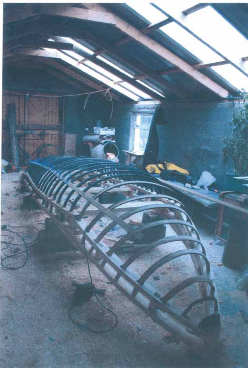
Figure 1. shows the frame and the internal structure of the hull of the currach. The internal hoops or “lats” are made of oak.
