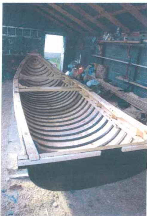
Figure 8. The currach receives two coats of resin mixed with a black pigment to bring her to the finished condition.
