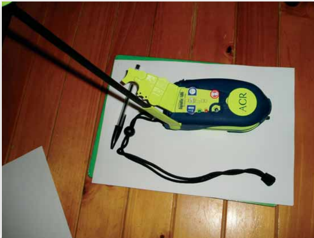
PLB with Flap open and aerial in extended position.
