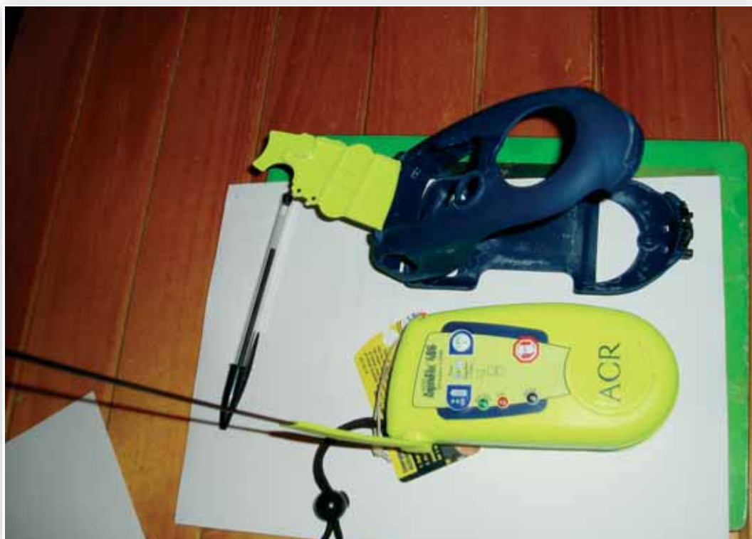
PLB Removed from Housing.
