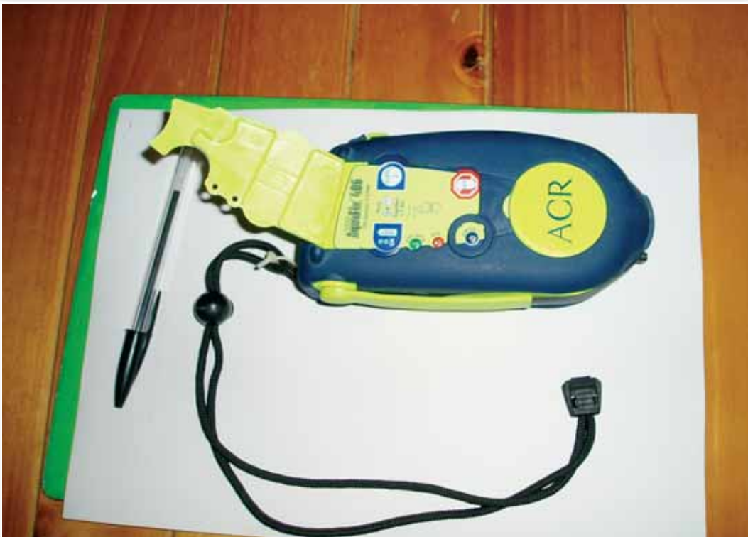
PLB with Flap open showing operating buttons. Test and GPS (Aerial in housed position).
