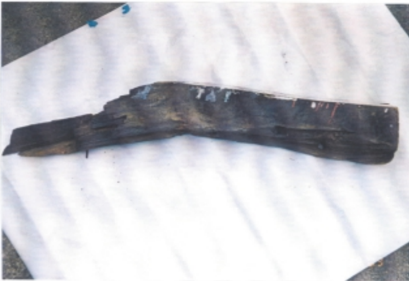
Figure 3. Frame 2. Grain running along axis of arms.
