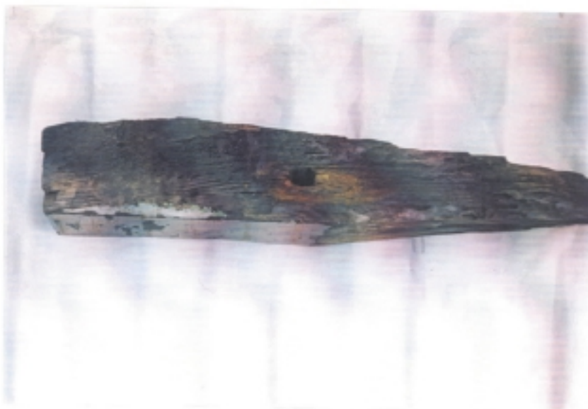
Figure 1, Frame 1. Surface soft rot to left of hole. Insect attack at extreme right.
