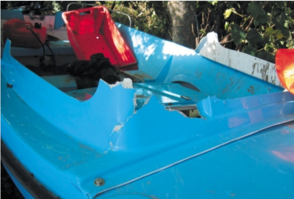
The Sullivan 460 viewed from forward with the fishbox used for storing the PFD's aft. Note the damaged section of the cuddy.
