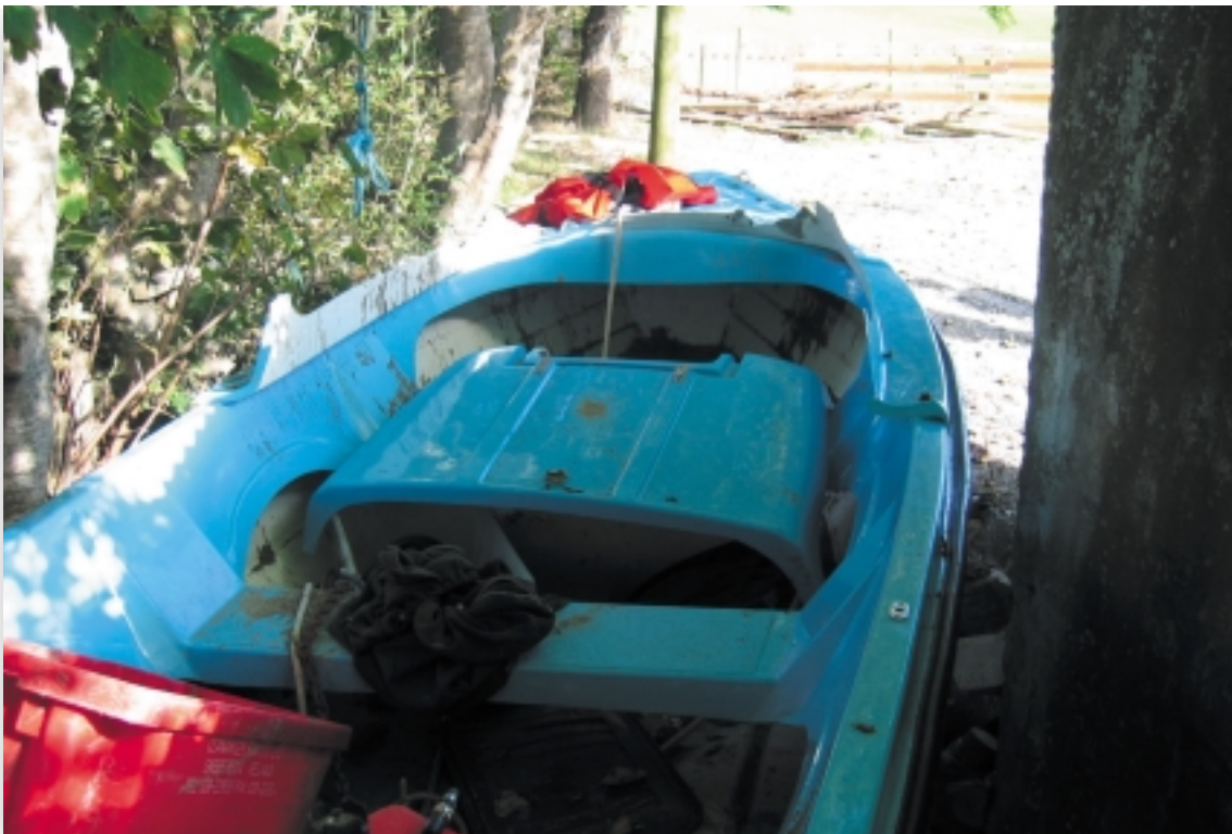
Sullivan 460 from stern with damaged cuddy in the well of the boat.
