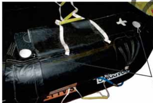
Repair patches applied FIGURE 8
