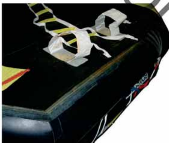
Throw over cylinder side of liferaft FIGURE 1
