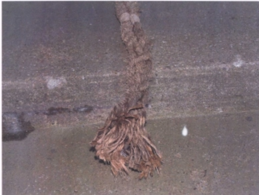
Photo 4 Close up of failure zone, Item A'
