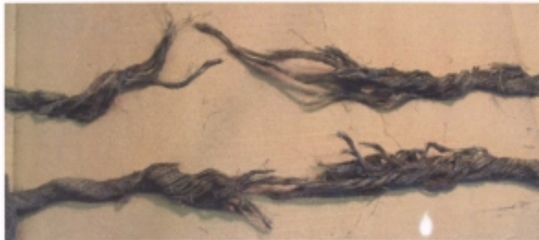
Photo 19 Typical tensile failures of rope strands
