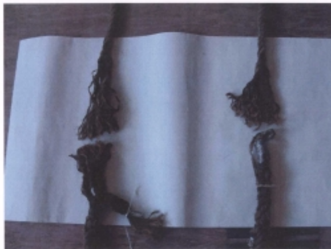
Photo 20 Failure zones of the ladder
