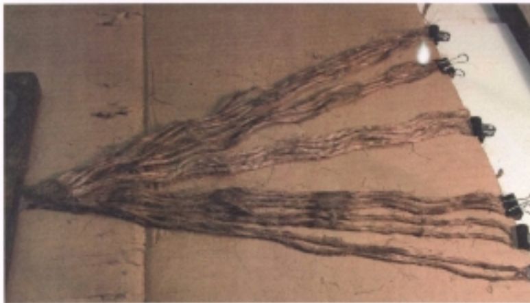
Photo 16 General view of unwound strand from ladder part Item A'
