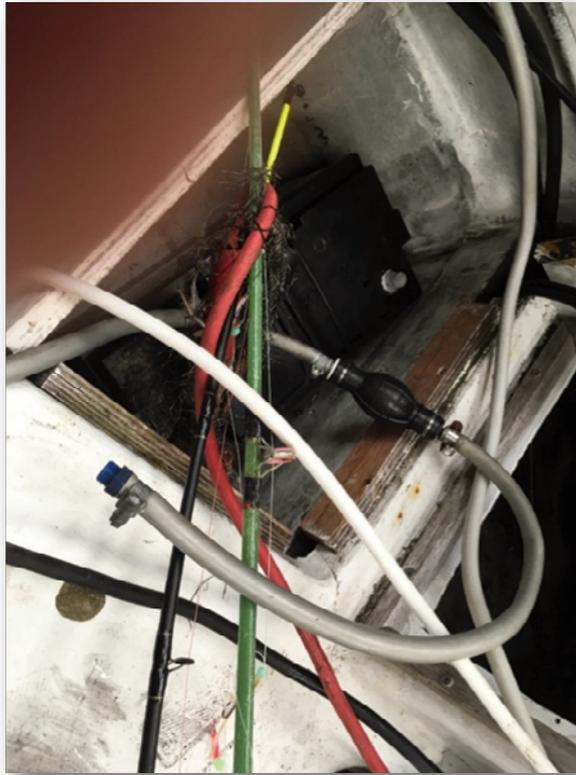
Photograph No.3 - *The threaded end of the fuel line & the spare battery.*
