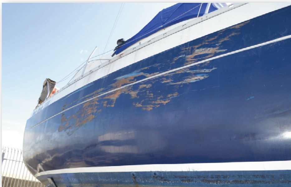
Photograph No.4 - Damage to hull, starboard side.
