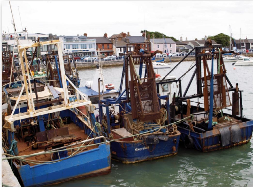
Photograph No. 3: Similar vessels showing the dredge in a stowed position on the gantry.
