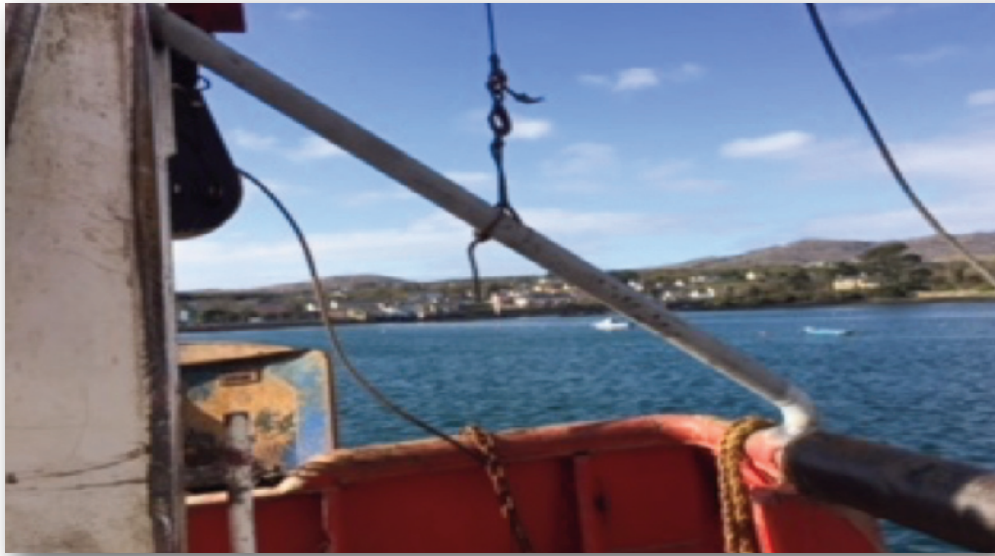
Photograph No. 4: Protection bars fitted.
