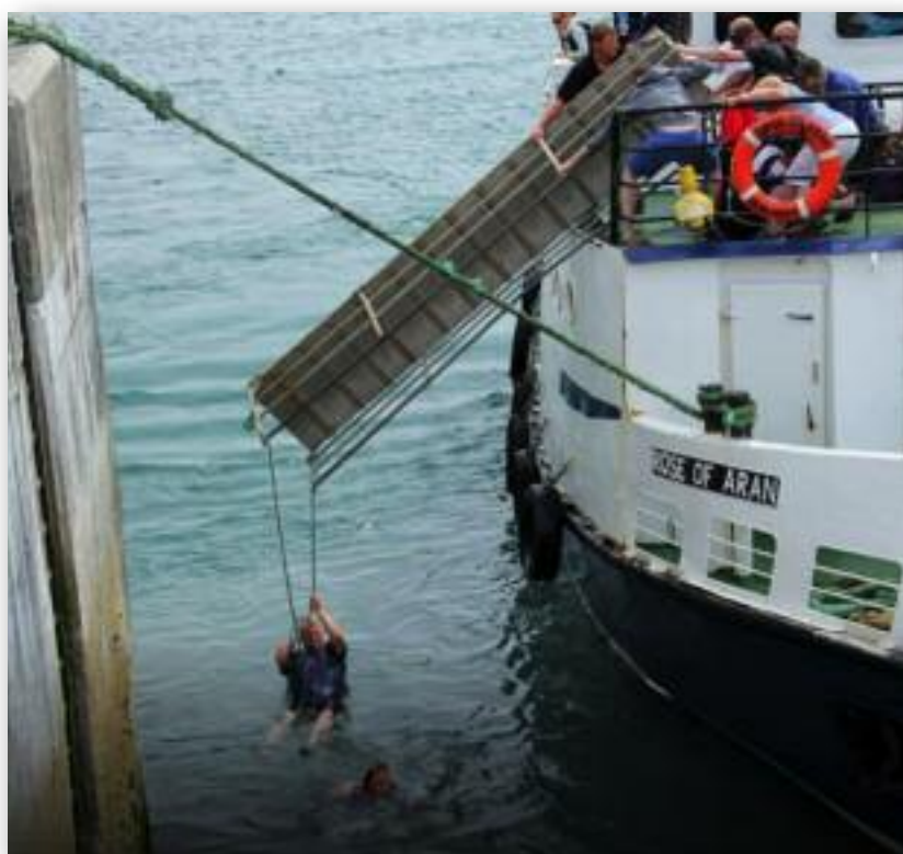
Photograph No. 4: The incident with gangway detached, one person swimming towards ladder and one person hanging on to gangway. Note no life-ring deployed at this stage, bow line and stern line have been taken back on board.
