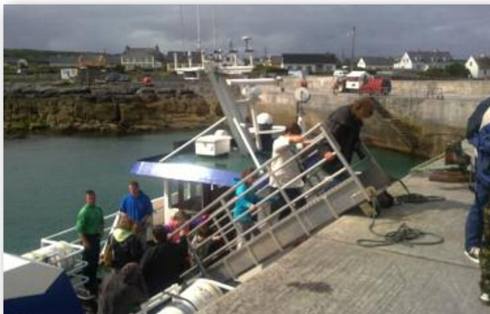
Photograph No. 2: Gangway from a ferry at Inis Oirr at low tide. Note steps from the pier on right hand side do not reach all the way to the water at this state of tide, also note marine growth at this level.
