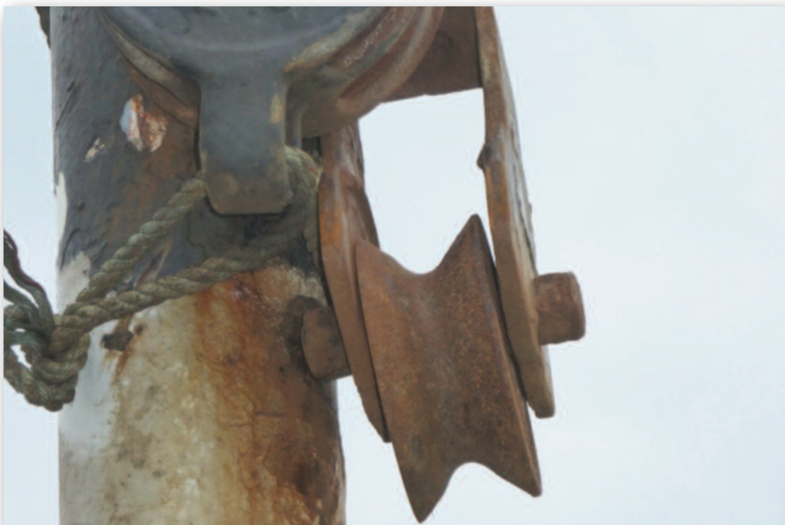
Photograph No. 6: Block at Derrick Head that Lazy Deckie, Split Links & Messenger Rope Passed Over
