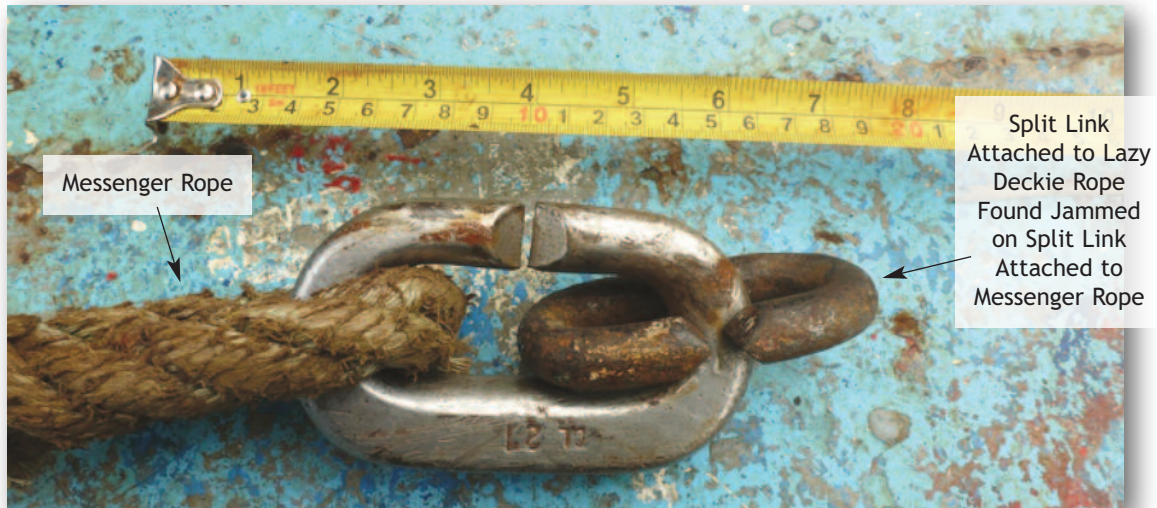
Photograph No. 3: Close-up of Split Links
