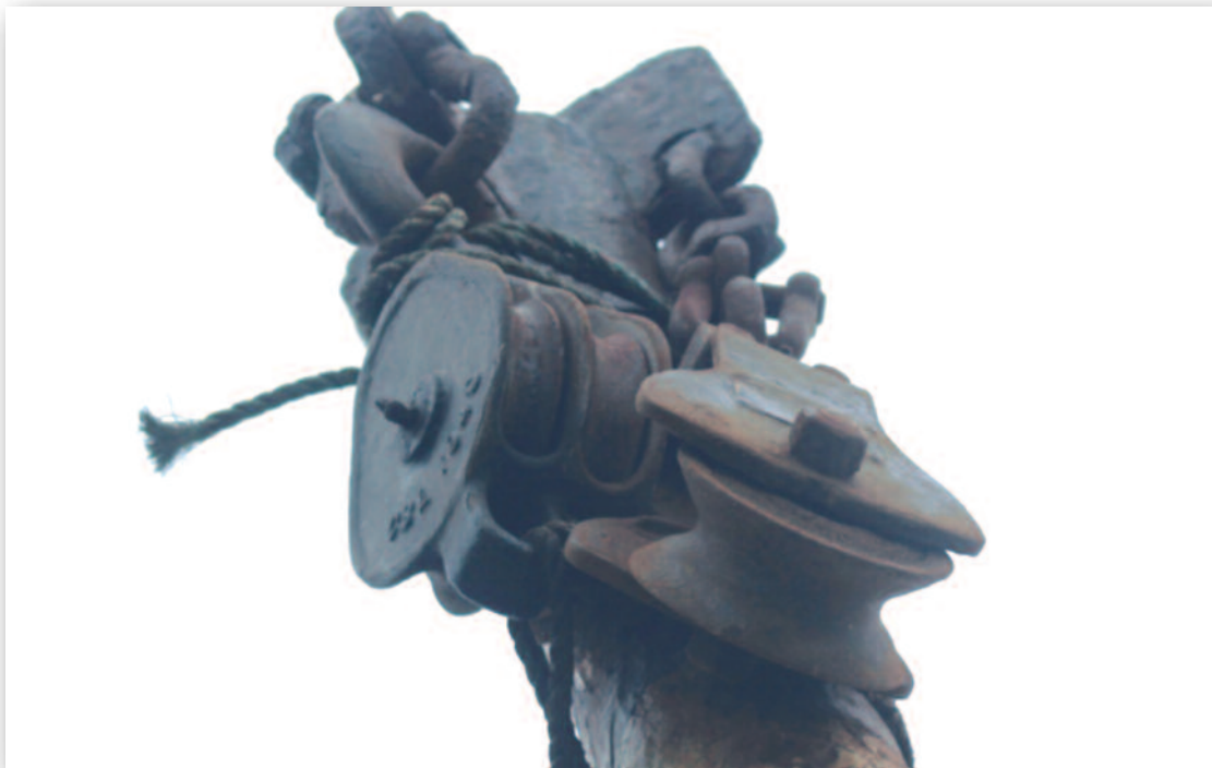
Photograph No. 5: Arrangement of Blocks on Derrick Head
