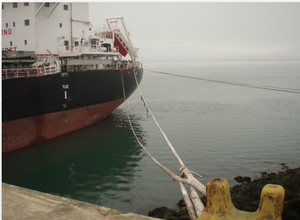
Photograph No. 5: View of after mooring lines - note all 4 lead in a forward direction.
