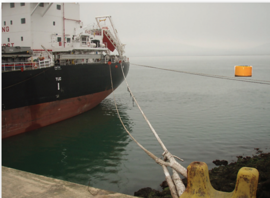
Photograph No. 6: Proposed large vessel mooring Buoy - this will be located Aft of the vessel so the after mooring lines will lead in an astern direction.
