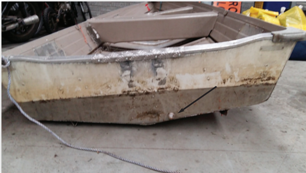
Photograph No. 1 - Transom of boat showing open drain hole.
