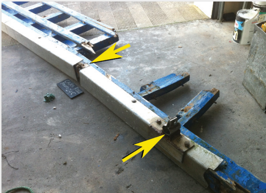
Photograph No. 6: Remains of Starboard Bulwark (inboard side) showing fracture point (upper arrow) - upper socket for pot hauler (lower arrow).
