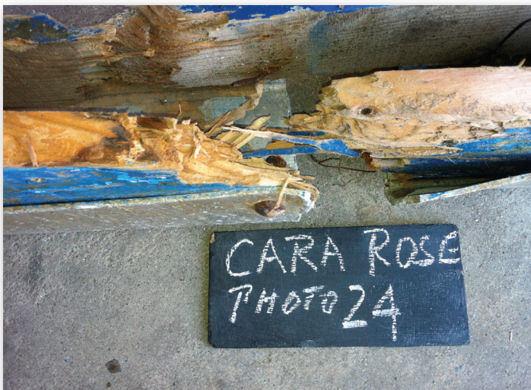
Photograph No. 8: Fractured bulwark wood - Splinters in outward direction.
