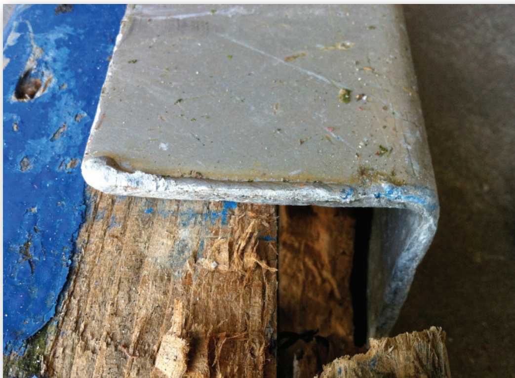
Photograph No. 7: Close up of fracture - note dull appearance of aluminium weld fracture.
