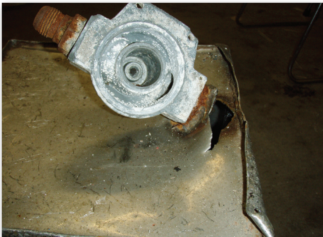
Photograph No. 10: Hydraulic oil reservoir for pot hauler - pipes torn off and steel torn by force.
