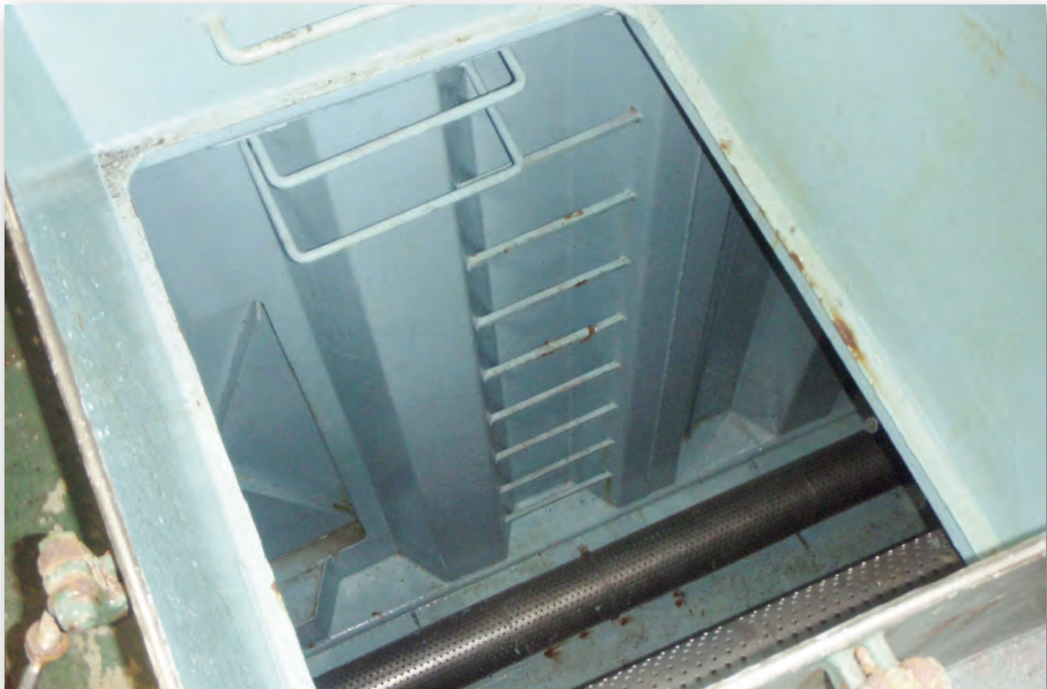
Photograph No. 4: Port Side Refrigerated Sea Water Tank.
