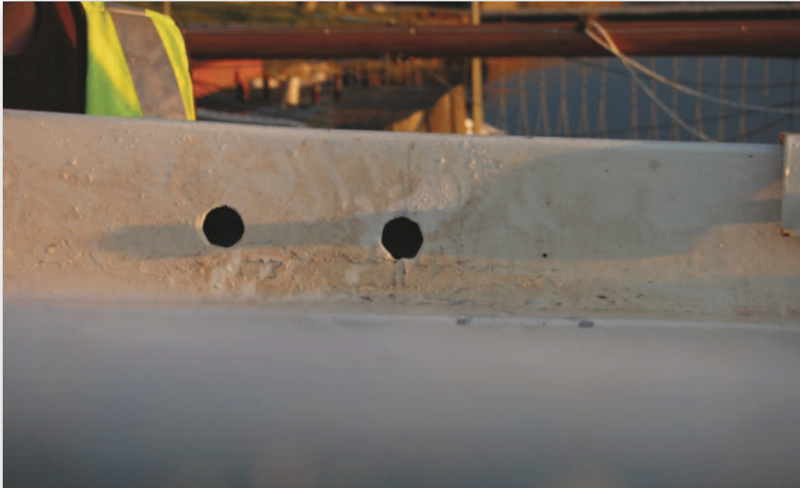
Photograph No. 5 - Picture showing holes cut in the inside of the gunwale
