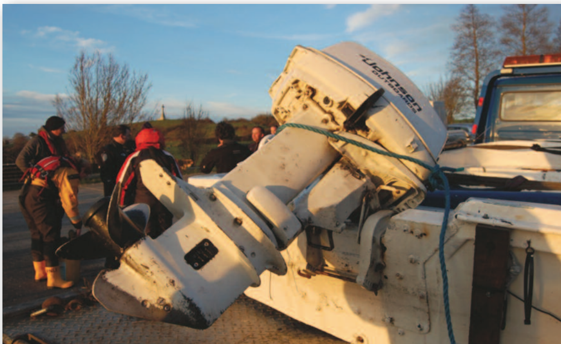
Photograph No. 3 - Transom of the boat draining water after the bung was removed
