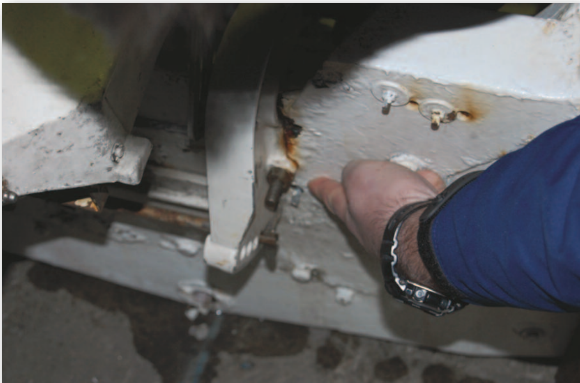
Photograph No. 6 - Transom with holes in the gunwale possibly from previous outboard motor brackets
