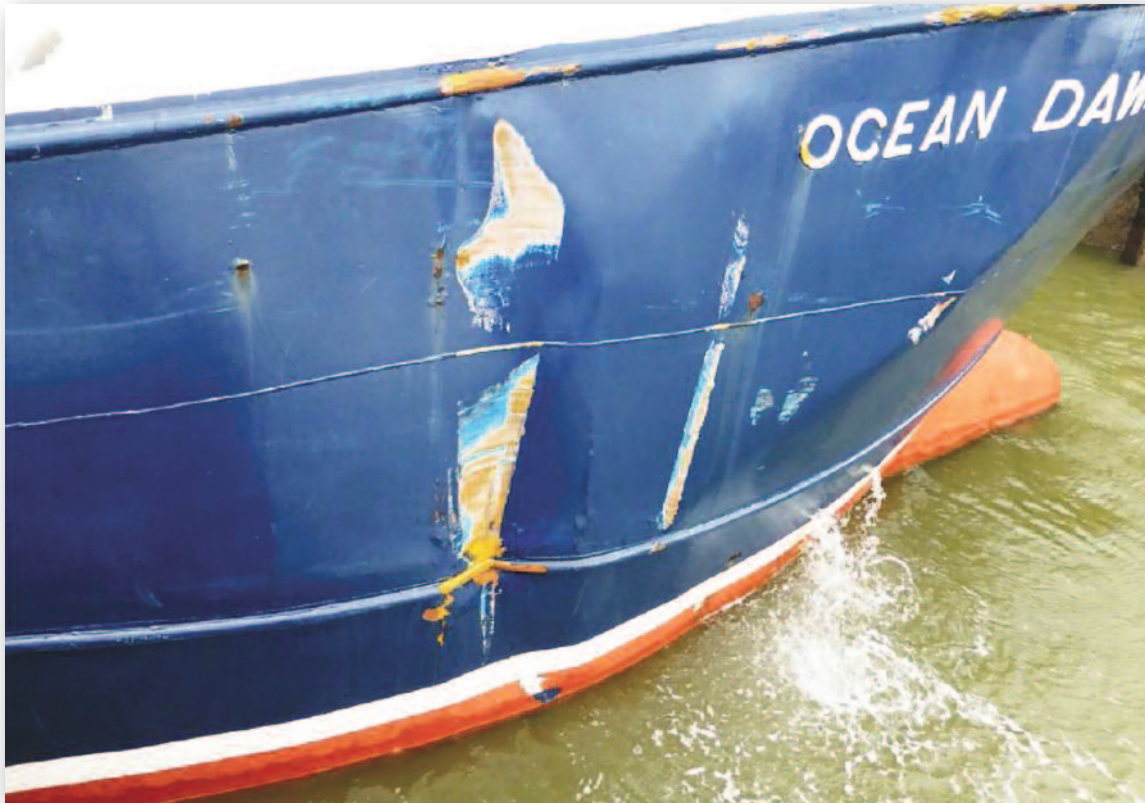
Photograph No. 13 - Damage to “MFV Ocean Dawn”
