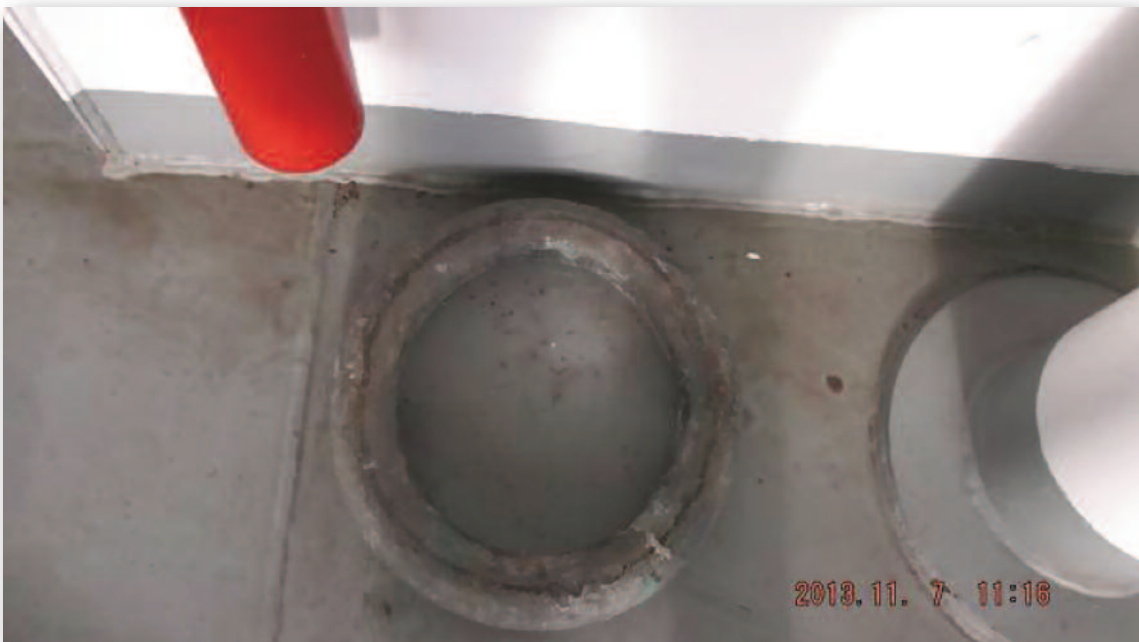
Photograph No. 4 - Mooring ring on deck, aft starboard side of accommodation area
