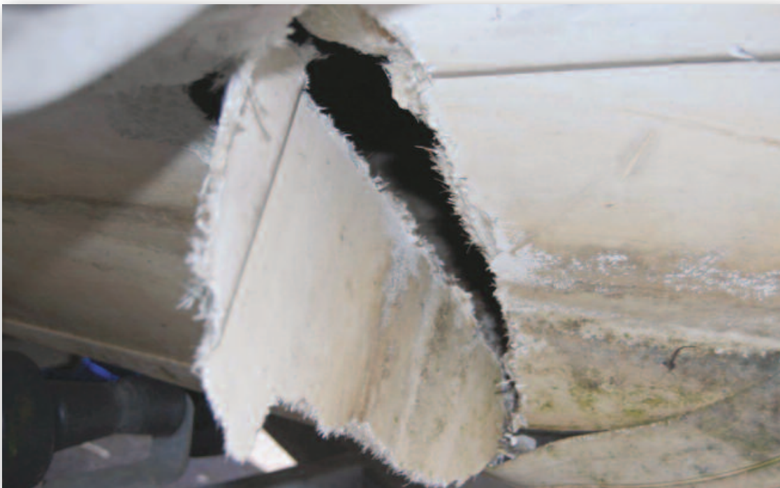
Photograph No. 4: Fold in the hull laminate on the starboard side
