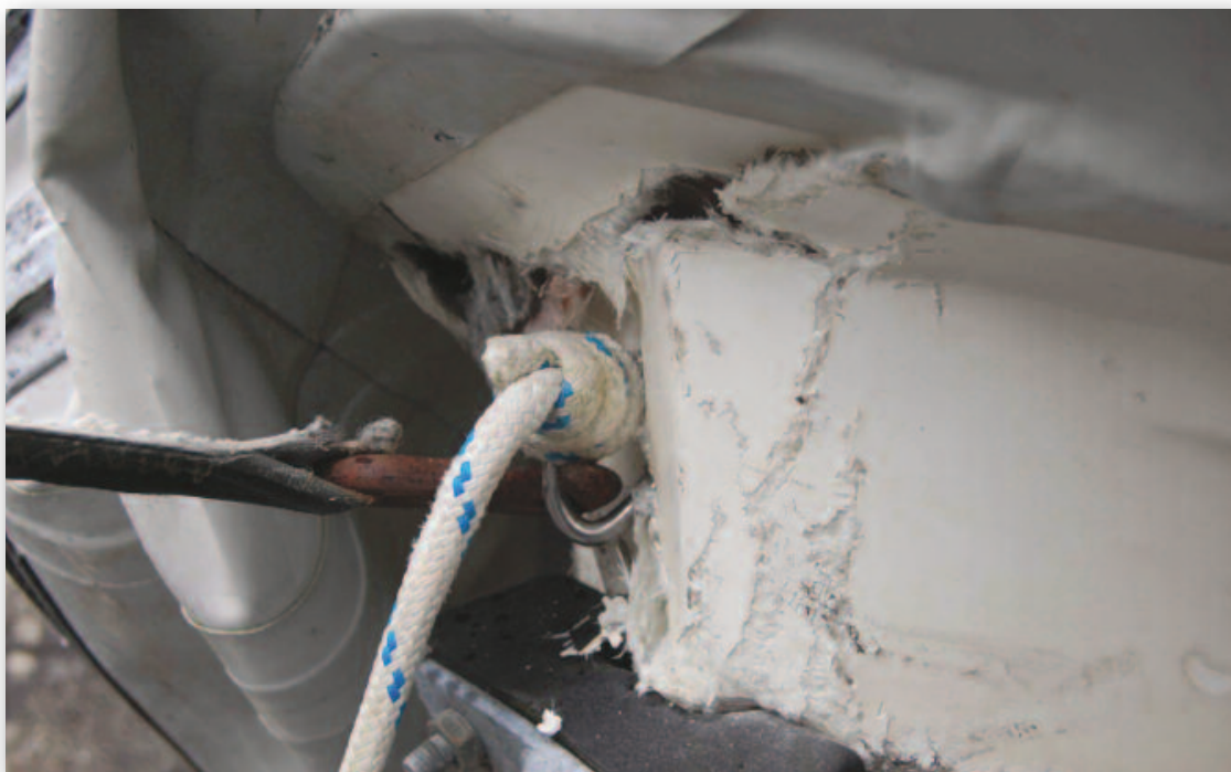
Photograph No. 2: Shows the smashed glass on the stem N.B. the rope is attached to the painter ring
