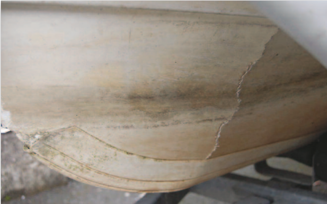
Photograph No. 3: Split in the hull laminate on the port side
