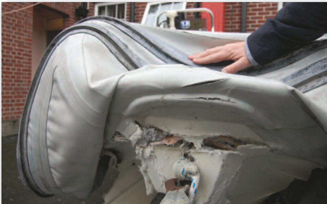
Photograph No. 1: Shows two of the tears that caused the forward chamber to deflate
