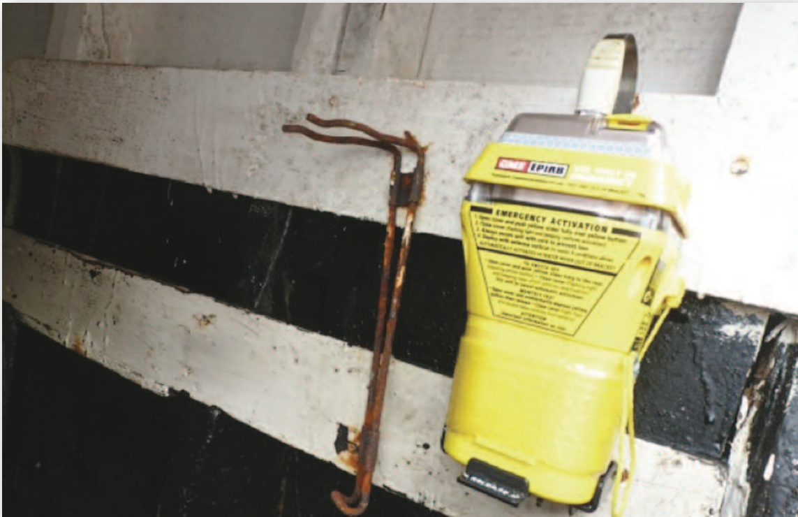
Photograph No. 5 - EPIRB Fitted in Holding Bracket Unlikely to come out of bracket without manual assistance from a person
