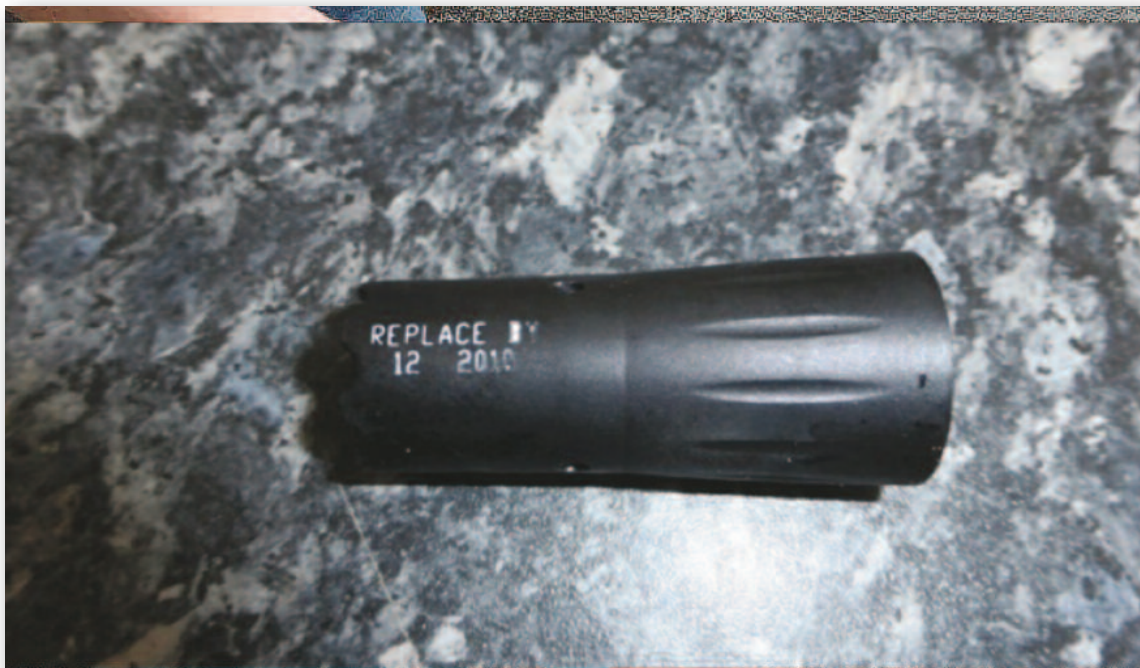
Photograph No. 15 - Hydrostatic Release on PFD From Casualty No. 3 Date indicates that it should have been replaced
