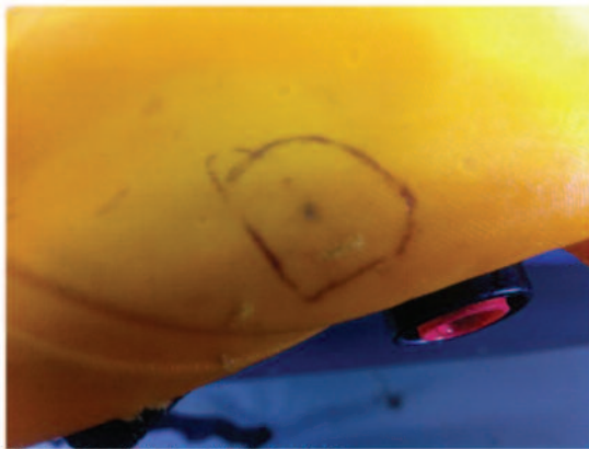
Fig. 2 - Small Holes Visible Jacket 1
