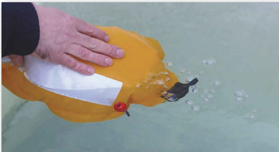
Photograph No. 14 - Leaking Bladder on PFD from Casualty No. 3
