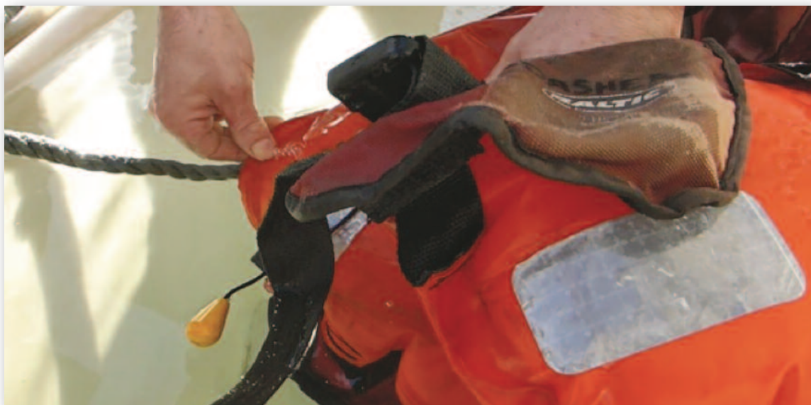
Photograph No. 13 - Leaking Bladder on PFD from Casualty No. 2
