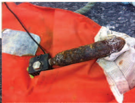
Fig. 4 Cylinder showing heavy corrosion
