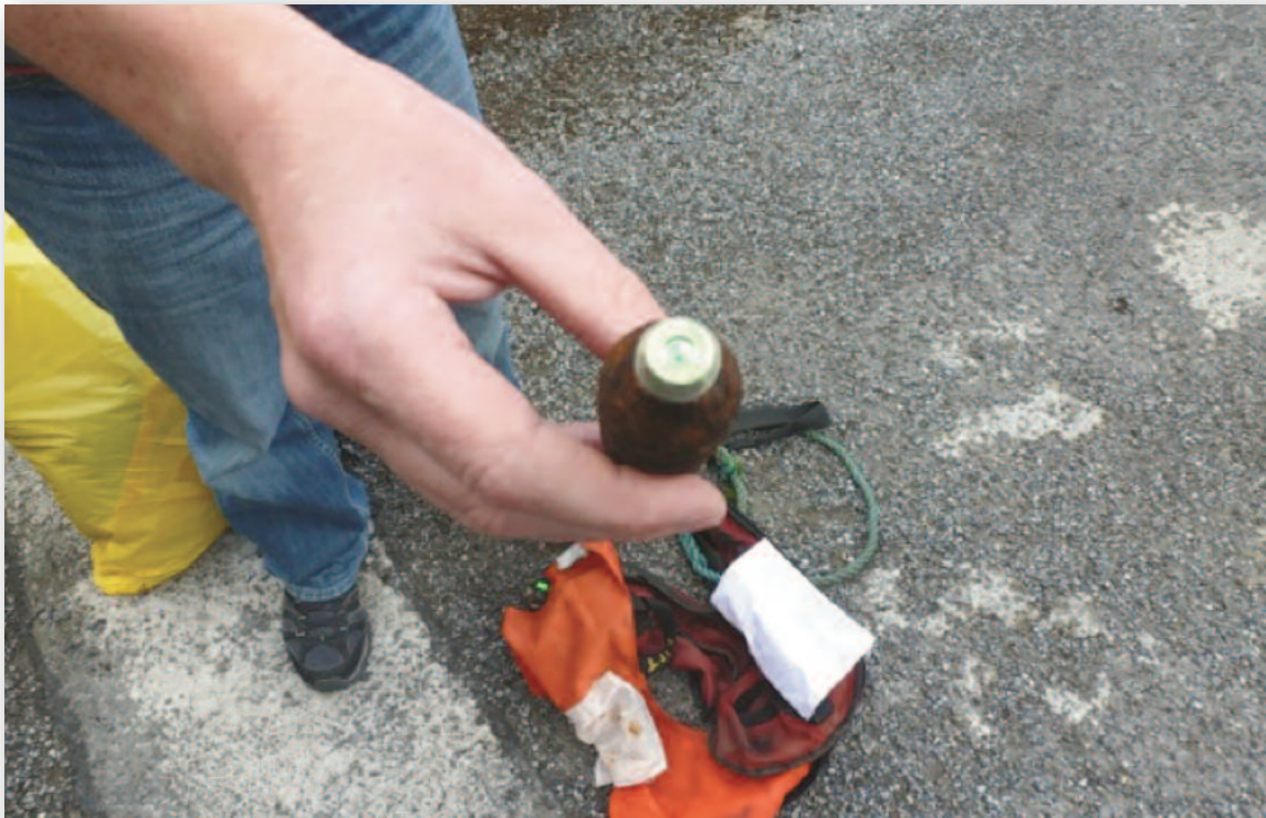
Photograph No. 12 - Seal on CO 2 Bottle Still Intact
