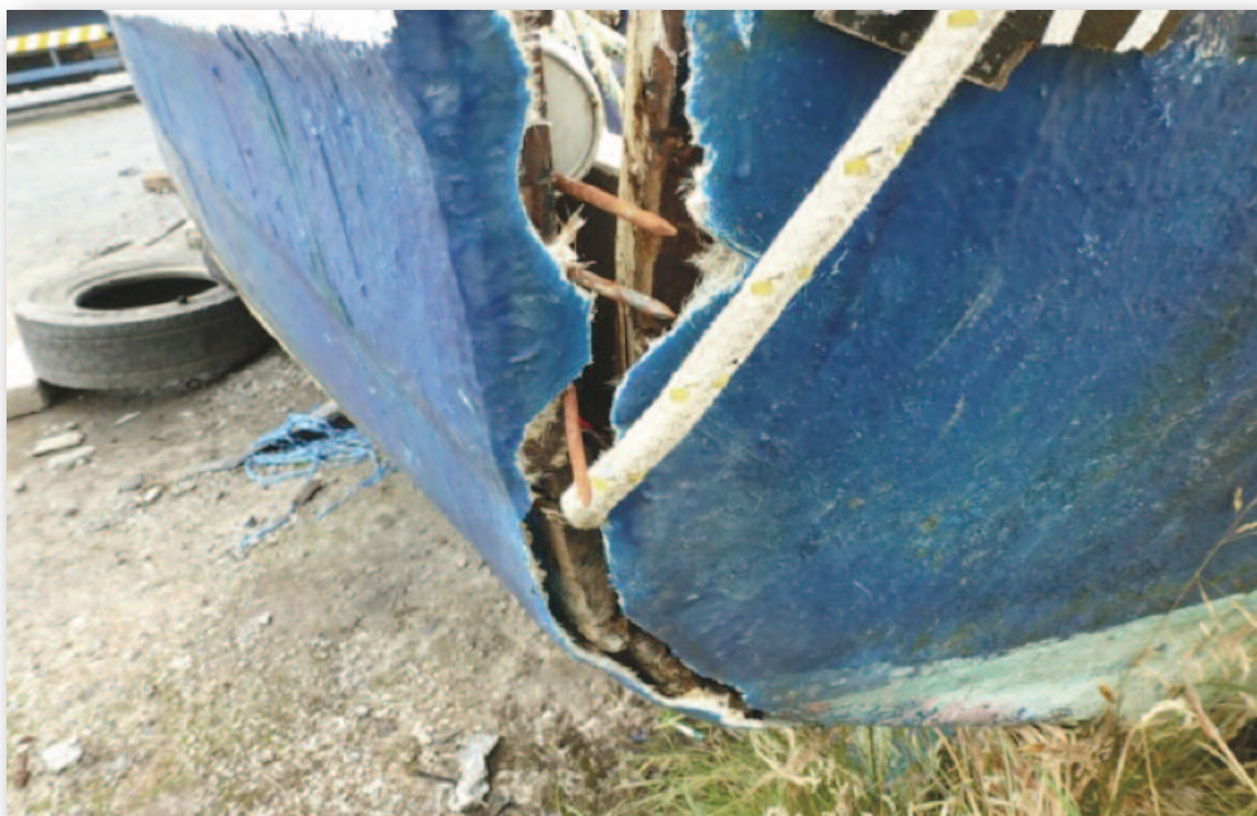
Photograph No. 2 - Damages to Transom
