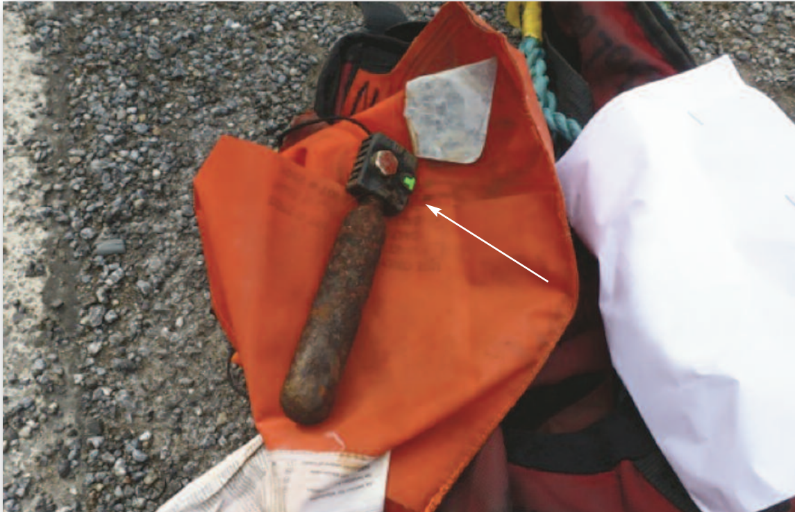
Photograph No. 11 - CO 2 Bottle in PFD Worn By Casualty No. 2 Note Tell-tale Indicates bottle Not Triggered.CO 2 bottle heavily corroded
