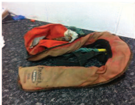
Fig. 3. Cover showing worn condition
