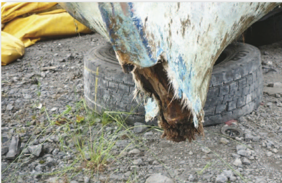
Photograph No. 4 - Damages to Stem
