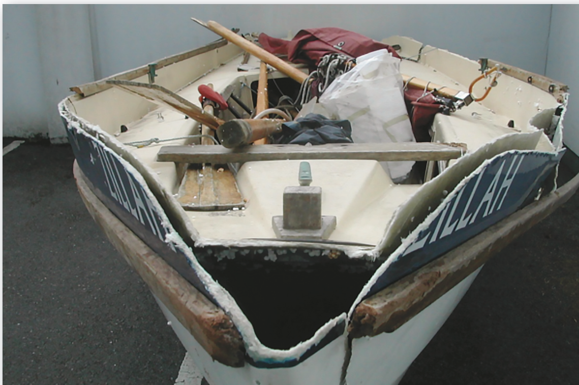
Photograph 2 - Damage suffered by "Zillah" following floundering
