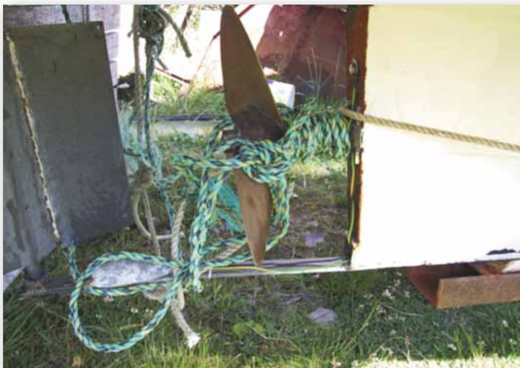
Photograph No. 2 - View of rope wrapped around propeller as seen at time of inspection
