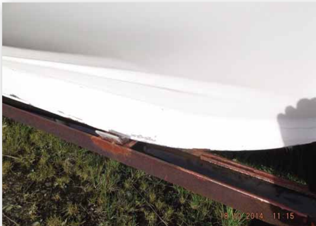
Photograph No. 5 - Shows cracking along keel line
