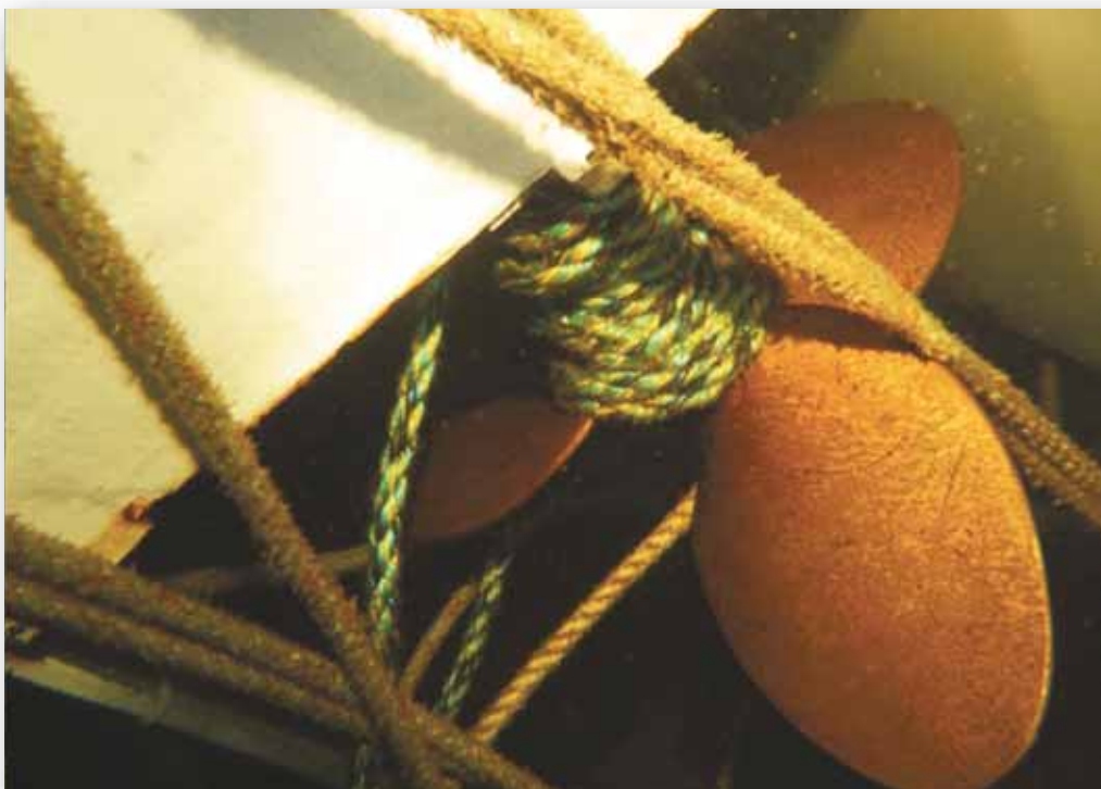
Photograph No. 1 - Underwater image showing rope wrapped around the propeller
